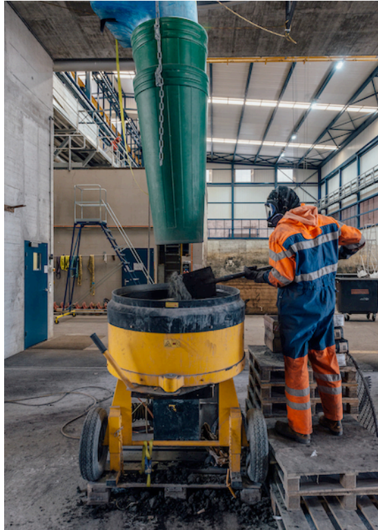
The waste is mixed with cement, lime, and pigment. Photo: Camilo Brau.
